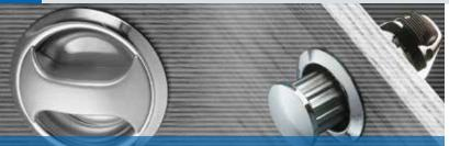
Southco's Push-to-Close latches simply slam shut, and do not require secondary steps for latching. The mechanism is mounted inside the enclosure, concealing latch points for enhanced security and aesthetics. Visible mounting styles provide actuation capability as well as a convenient handgrip for opening the door or panel.
